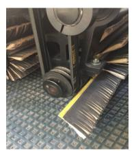
cupboard or bottom of carving door, which is bring polishing function into full play. the Oscillation power is 1/4HP  $\times$  4
