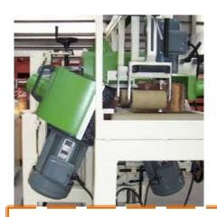
Each Left and Right sanding head can be adjust to Tilt forward
