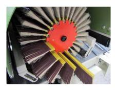
It's very easy and convenient to replace the brush wear strip on the hubs
