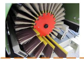
It's very easy and convenient to replace the brush wear strip on the hubs
