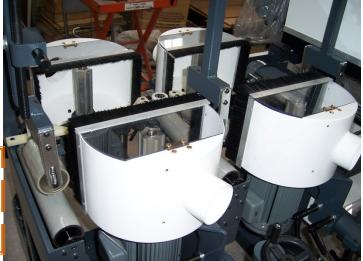
Each Left and Right sanding head can be controlled separately upward, downward, forward and backward.
