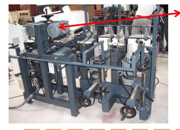
2 top and 2 bottom head , it is synchronous adjust to upward and downward.
