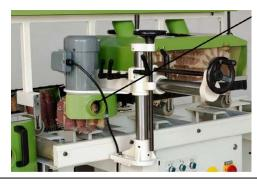
The location of all the sand head tilt can be adjusted to tilt
